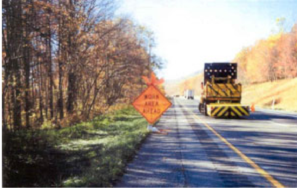
Photo 2. Truck equipped with a truck-mounted attenuator (TMA) and a lighted arrow signal.
